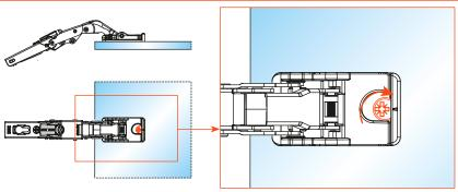
3) Rotate the fixing cam.
