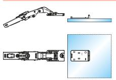
1) The hinge plate must be attached to the glass door with a specific adhesive using the correct procedure. We recommend that this operation is carried out by a specialist company. For further information on adhesives and their application, please contact the adhesive manufacturer or your glass supplier.
