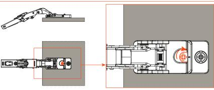
3) Rotate the fixing cam.
