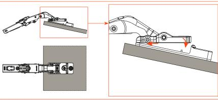
**2)** Locate the hinge onto the plate when it is fixed to the door.
